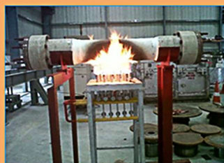
Fire Endurance Testing (IMO Level 3)
